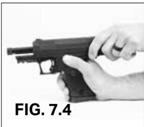
4. Lock the slide in the rearward (open) position by pushing the manual safety/manual slide lock up into the notch on the slide and slowly releasing the slide from the fully rearward position until it locks in the open position. (Fig. 7.4)
