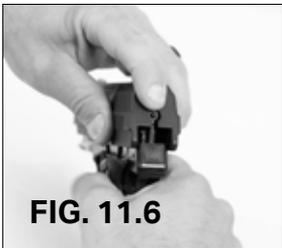
6. Pull the slide back toward the rear of the frame until the slide retainer is aligned with the hole at the rear of the frame (FIG. 11.6) and slide it back enough to clear the firing pin from hitting the barrel if it is protruding from the breach face. Then push the slide down to lock it back in place. (Note: If necessary, use the index finger of your firing hand to guide the slide retainer down and into the hole in the rear of the frame.)
