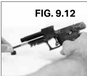
11. Pull the recoil spring and recoil spring guide rod forward and out of the frame. (Fig. 9.12)
