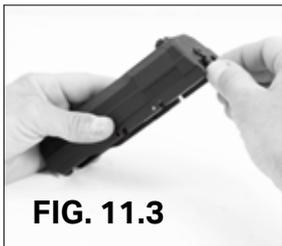
3. Install the slide retainer into the slide by holding the cylindrical part and inserting the rounded part into the channel at the rear of the slide. (FIG. 11.3)
