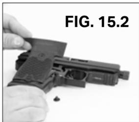
3. Use the dual lok wrench/adjustment tool or a small flat screwdriver to pry the grip panel up and away from the frame. (Fig. 15.2)
