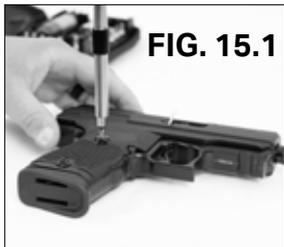
1. Make sure that the magazine is removed and the manual safety is fully upwards in the on (safe) position.
