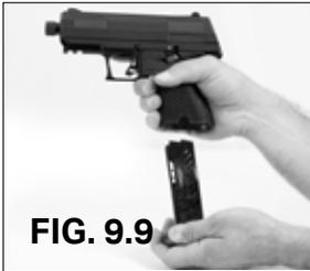
8. Insert an EMPTY magazine into the magazine well to deactivate the magazine disconnect device and, with the muzzle of your Hi-Point pistol pointed in a safe direction (a safe direction is one in which no one can possibly be injured in the event of an unintentional discharge), pull the trigger to release the striker. (Note: Although it is possible to disassemble your Hi-Point pistol with the striker cocked, it is much easier to remove the slide with the striker released.) (Fig. 9.9)
