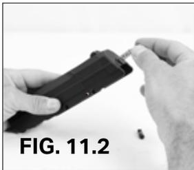
2. Install the firing pin spring and firing pin assist spring into the slide by holding the slide with the muzzle facing down and sliding the firing pin spring and firing pin assist spring down and into the channel in the rear of the slide. (FIG. 11.2)
