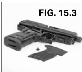
4. Lift the grip panel up and away from the frame. Note: Removing the grip panel exposes parts inside the frame. Be careful not to remove/dislodge them. (Fig. 15.3 & 15.4)
