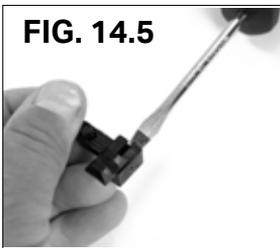
6. Align the round opening on the bottom of the new rear sight against the opening on the left side of the adjustable rear sight assembly and push it against the windage screw. Turn the windage screw clockwise with the dual lok wrench/adjustment tool or a small flat screwdriver until the new sight is centered in the adjustable rear sight assembly. (Fig. 14.6)
