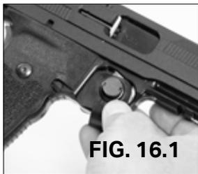
1. Remove magazine before installing the Dual Lok. Align the Dual Lok so that the strap is underneath the trigger guard with the lock head on the right side (the side with the ejection port) of the pistol. (Note: The Dual Lok must be installed with the lock head on the right side to fit properly).
