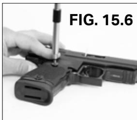
7. Install the grip screw by turning it clockwise using a 1/8" allen wrench/driver. Do not overtighten grip screws, snug is sufficient. (Fig. 15.6)
