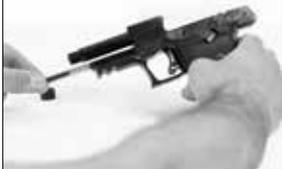
4. Install the recoil spring and recoil spring guide rod into the frame by pushing them into the cylindrical area of the frame below the barrel with the guide rod facing forward. (FIG. 11.4)
