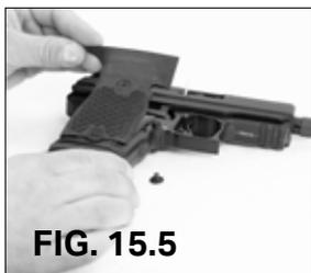
6. Press the top of the new grip panel down against the frame until it snaps into place.
