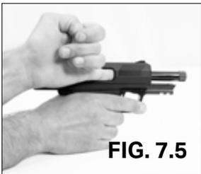
5. Once the slide is locked to the rear, visually and physically (with your finger) inspect the chamber and the magazine well of your Hi-Point pistol to be sure that no ammunition remains in either place. (Fig. 7.5)
