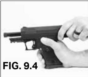
4. Lock the slide in the rearward (open) position by pushing the manual safety/manual slide lock up into the notch on the slide and slowly releasing the slide from the fully rearward position until it locks in the open position. (Fig. 9.4)
