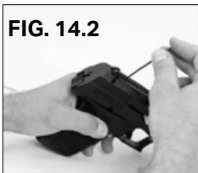
2. Use the dual lok wrench/adjustment tool or a small flat screw driver to remove the elevation screw by turning it counterclockwise. (Fig. 14.2)
