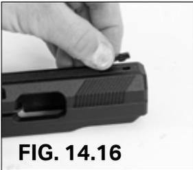
2. With an upward motion, remove the front sight from the slide. (Fig. 14.16)
