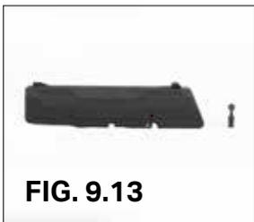
12. Pull the slide retainer out the back of the slide. (Fig. 9.13)
