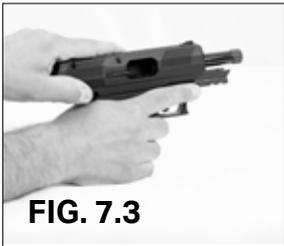
3. Ensure the ejection port is facing away from you and the pistol is pointed in a safe direction (a safe direction is one in which no one can possibly be injured in the event of an unintentional discharge). While holding the grip with your firing hand and with your finger off of the trigger and outside of the trigger guard, grasp the rear of the slide at the serrated area with your other hand and pull the slide fully back to eject any cartridge that may be in the chamber. (Fig. 7.3)
