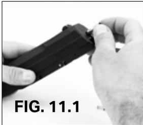
1. Install the firing pin into the slide by holding the slide with the muzzle facing down and sliding the firing pin down and into the channel in the rear of the slide. (Fig. 11.1) Verify firing pin moves freely and protrudes the breach face with no restrictions.
