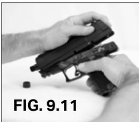
10. While holding a finger over the rear of the slide pull the slide approximately 3/8" to the rear and then pull the rear of the slide up and push it forward to remove the slide assembly from the frame.
