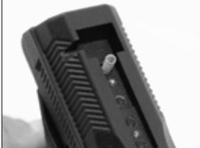
7. Place the adjustable sight spring into the round hole at the top of the slide. (Fig. 14.6)
