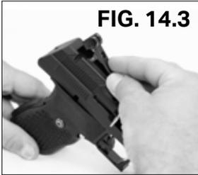
3. Carefully lift the adjustable rear sight assembly up and away from the slide. (Fig. 14.3)
