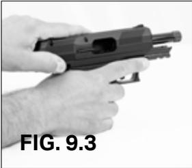
3. While holding the grip with your firing hand, with your finger off of the trigger and outside of the trigger guard, grasp the rear of the slide at the serrated area with your other hand and pull the slide fully back to eject any cartridge that may be in the chamber. (Fig. 9.3)
