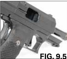
5. Once the slide is locked to the rear, visually and physically (with your finger) inspect the chamber and the magazine well of your Hi-Point pistol to be sure that no ammunition remains in either place. (Fig. 9.5)
