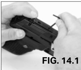
1. Use the included 3/32" Allen wrench to remove the sight pivot retainer screw by turning it counterclockwise. (Fig. 14.1)
