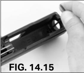
1. Using a 5/64" hex key, remove the front sight screw and nut. (Fig 14.15)
